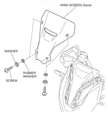
2. Install the wind screen of the accessory in reverse order of the removal.
